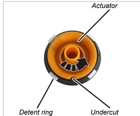
→ Turn the actuator of the new push-button cap so that the undercut lies precisely between two catches.
