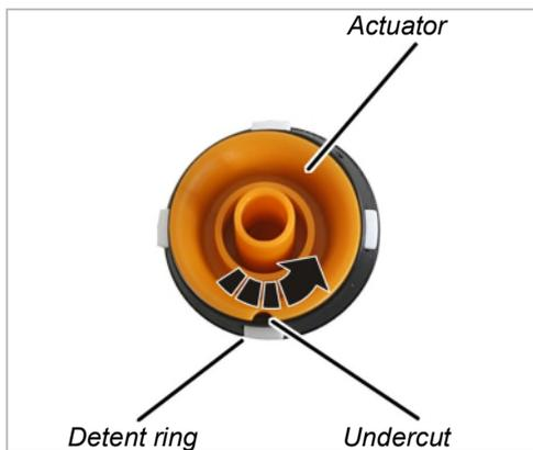
→ Turn the actuator of the new push-button cap so that the undercut lies precisely against one of the catches.
