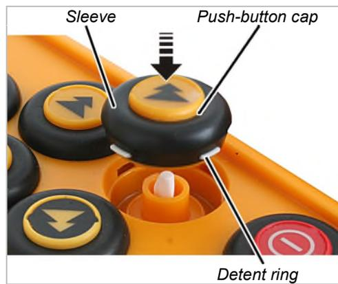
→ Attach the new push-button cap. The undercut ensures that the cap fits in only a single position.
